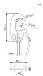
Works on diameters from 20mm to 55mm.
